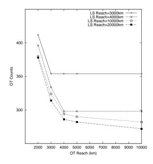
Figure 6: OT counts for varying OT reaches and line system length limits. When the OT reach is longer than the line system limit, OT counts cannot be reduced further no matter how big OT reach is.
